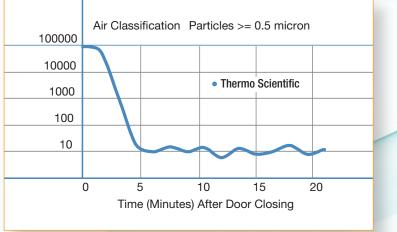
Security for your cells. The HEPA filter provides a 4 log reduction of particles in 5 minutes. ISO 5 clean room air quality achieved in 5 minutes from a door opening.
