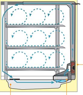
Incoming air first travels over a direct heated water reservoir resulting in 50% faster humidity recovery than with a standard water pan design.\*\* The in-line HEPA filter cleans the airstream of microbes and particles protecting cultures from contamination.
