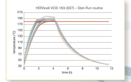
Pharmacopeias no longer recommend a given temperature and time for sterilization. Instead, they require proof of performance. During Steri-Run, all chamber surfaces are proven to reach sterilization temperature.
