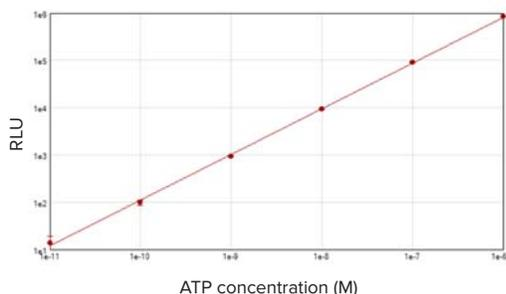
**An ATP standard curve spanning five decades was run using the ATPlite 1step Luminescence Assay System (PerkinElmer) on the SpectraMax iD3 reader.** Standard concentrations ranged from  $1 \times 10^{-11}$  M to  $1 \times 10^{-6}$  M. A wide linear dynamic range ensures accurate assay results across a broad span of sample types. Standards were plotted using a log-log curve fit in SoftMax Pro Software.
