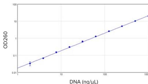
**The SpectraMax iD3 reader is fully compatible with the SpectraDrop™ Micro-Volume Microplate, enabling quantitation of precious low-volume samples.** 4-μL DNA standards from 2 ng/μL to 1000 ng/μL were read in absorbance detection mode with a preconfigured protocol in SoftMax Pro Software. Performance matching the 2 ng/μL sensitivity specification is demonstrated here.
