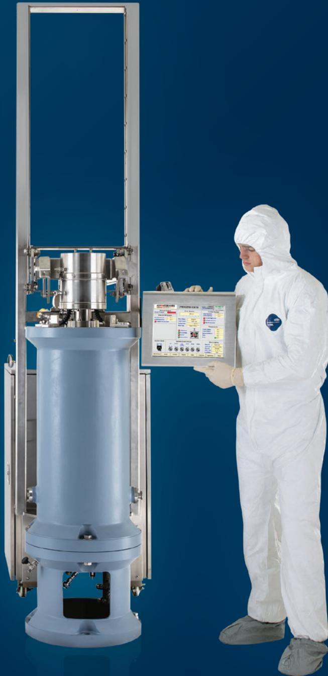
The KII system is designed to expertly perform in FDA approved processes for the manufacture of viral vaccines, particulate proteins, gene therapies and nanostructures.
