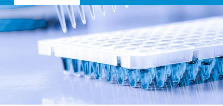
Labmore  $^{\circledR}$  filtered pipettes tips are designed to fit volumes ranging from 0.1  $\mu L$  to 1,250  $\mu L$  and can efficiently draw and deliver required liquids in any application with high levels of accuracy and precision.
