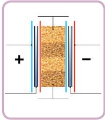
Electrodeionization, EDI, unites two proven technologies for producing ultrapure water: Electrodialysis and ion exchange. In contrast to conventional ion exchange in which resins must be either chemically regenerated or the cartridge discarded, EDI utilizes an electric current for continual resin regeneration.
