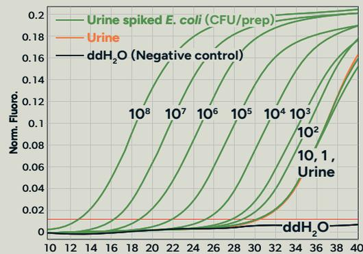
The extracted DNA from urine by FAUD103 in qPCR analysis demonstrated favorable performance for wide-range sample inputs and effectively removing PCR inhibitor.
