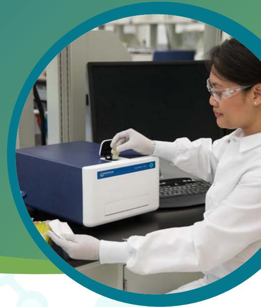
The SpectraMax® ABS Microplate Reader bridges the gap between the affordability of filter-based readers and the flexibility of monochromator-based systems.
