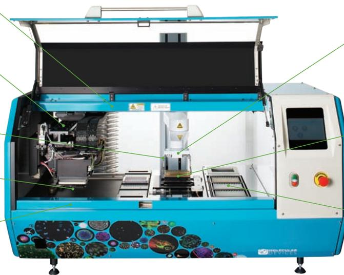
Acoustic sensors detect agar height, helping high-precision robotics to **pick single colonies gently and accurately**
