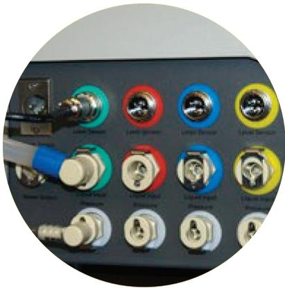
**Figure 2. Color-coded inlet connectors.** Color-coded inlets with quick connects decrease assembly time and allow the use of multiple buffers and solutions without bottle switching. The level sensors, when connected to the reservoir bottle sensors, detect if bottles are empty or full.
