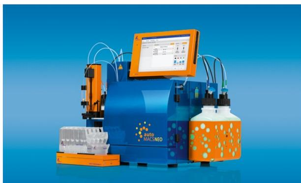
**Figure 3:** The full setup of the autoMACS NEO Separator.
