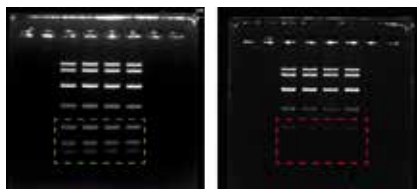
Detection of small bands using high quality FastGene® Agarose and Competitor C's Agarose. All seven bands from the ladder are visible when using FastGene® Agarose. When comparing the green box to the red box, Competitor C's Agarose does not show the lowest three bands.
