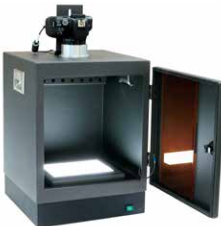
Position the white LED illuminator in the central area and adjust the recording settings in the NIPPON Genetics Camera Studio.
