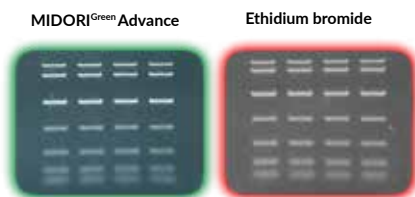
Comparison of sensitivity between MIDORI Green Advance and ethidium bromide using a UV-transilluminator.
