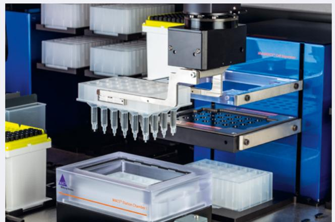
**Figure 10:** The MultiMACS X is equipped with a gripper arm and a 4-tip liquid handling arm for maximal flexibility and reliability with different applications.
