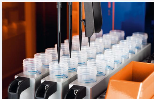
**Figure 8:** Cooled Chill Racks keep the samples and reagents at 2–8 °C.
