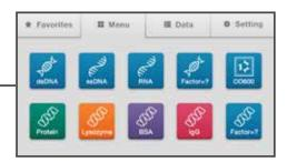
The software of the EastGene® NanoView was made for easy handling. The main menu tab enables easy navigation through distinct measurement modes via touchscreen with intuitive icons
