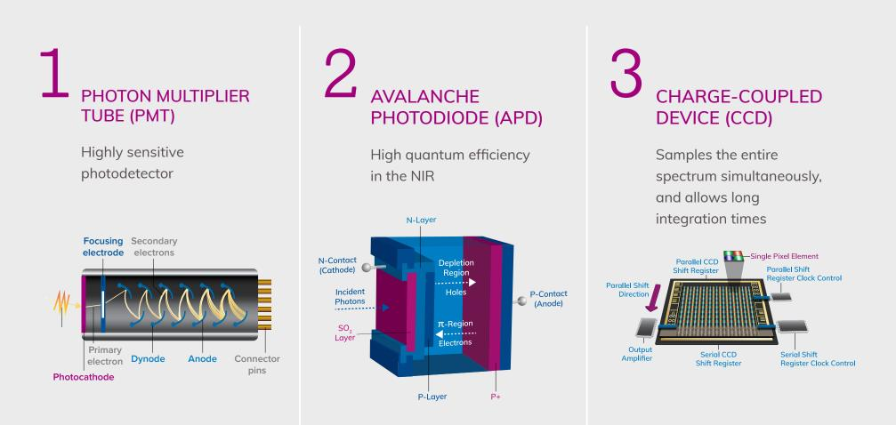
The Sapphire Biomolecular Imager's patent pending design uses 3 different detection modes to deliver ultimate application flexibility. Using PMTs, APDs, and CCD, the Sapphire is a unique system designed for visible fluorescence, NIR fluorescence, and chemiluminescent imaging.
