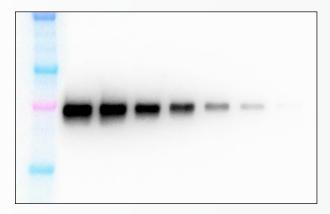
Simultaneous imaging of chemiluminescent samples and colored molecular weight markers. Images are captured serially, and then overlaid within the capture software.
