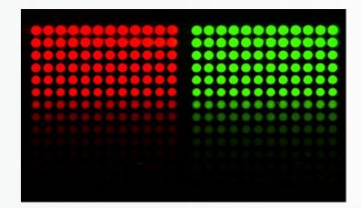
Full Moon BioSystems Scanner Calibration Slide scanned at 10 µm resolution using the 520 nm and 658 nm channels of the Sapphire Biomolecular Imager.
