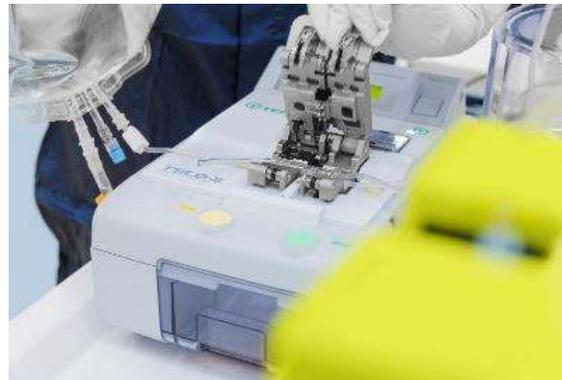
*Tubing set compatible for sterile welding*
